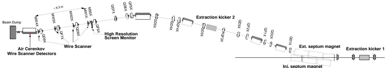
Fig. 1 Layout of the ATF-DR extraction line
