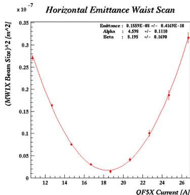
Fig. 5 Waist scan plot in X using QF5X
