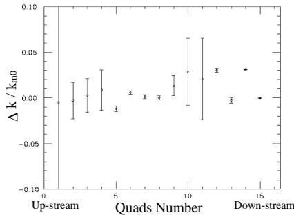
Fig. 2 Fitted relative errors of quads k-values
