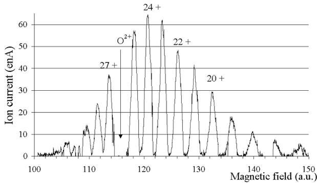
Figure 1:  $Pb^{n+}$  spectrum for a 65 nAe  $Pb^{1+}$  injected beam
