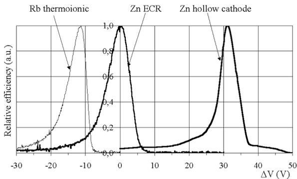
Figure 3: Variation of the relative efficiency versus  $\Delta V$
