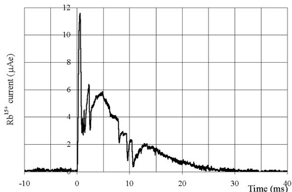
Figure 6: 400 nA  $\text{Rb}^{1+}$  injected; 11.5  $\mu\text{Ae}$   $\text{Rb}^{15+}$  extracted
