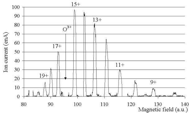
Figure 2:  $Rb^{n+}$  spectrum for a 135 nAe  $Rb^{1+}$  injected beam
