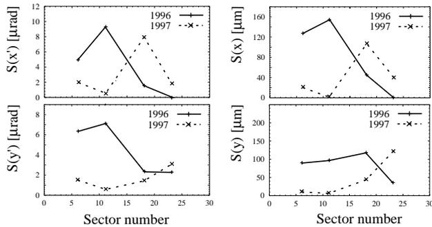
Figure 4: RMS variation  $S$  of the different feedback setpoints  $x'$ ,  $y'$  (left) and  $x$ ,  $y$  (right) over three month periods in 1996 and 1997. The feedback position and angle offset introduce trajectory oscillations (= emittance bumps) up to the next feedback. The electron and positron setpoint variations are averaged. The bias towards later bumps is clearly seen for the new 1997/98 tuning approach.
