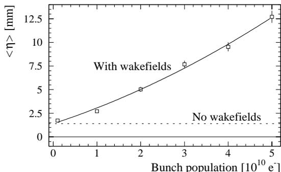
Figure 2: Expected dispersion  $\langle \eta \rangle$  in the end of the SLC linac as simulated for different SLC bunch currents. The wakefield-free dispersion is indicated by the dotted line. The SLC linac dispersion is driven by wakefields.
