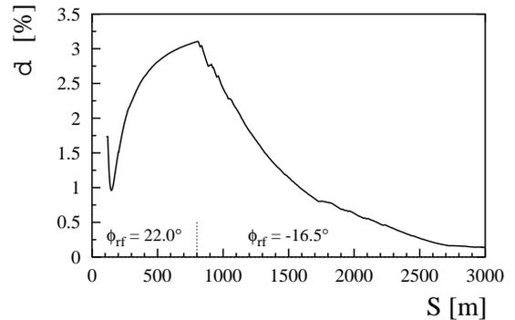
Figure 1: Typical BNS relative energy spread  $\delta$  along the SLC linac.
