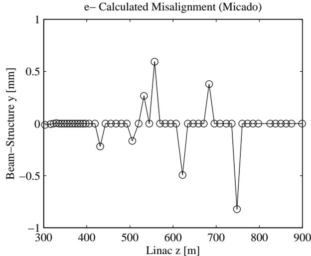
Figure 2: Calculated structure misalignment from observed difference orbit for different bunch length.
