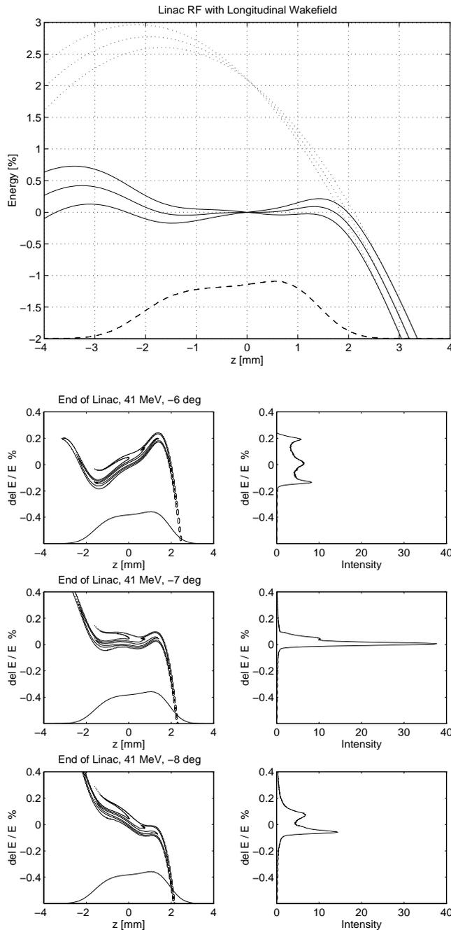
Figure 4: Energy– $z$  correlation for different linac phase.
