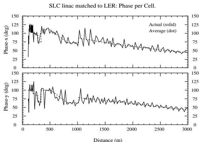
Figure 1: Phase advance of the  $110^\circ/\text{cell}$  SLC lattice.
