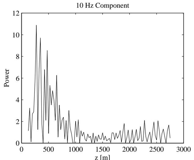
Figure 3: 10 Hz line plotted along the linac.
