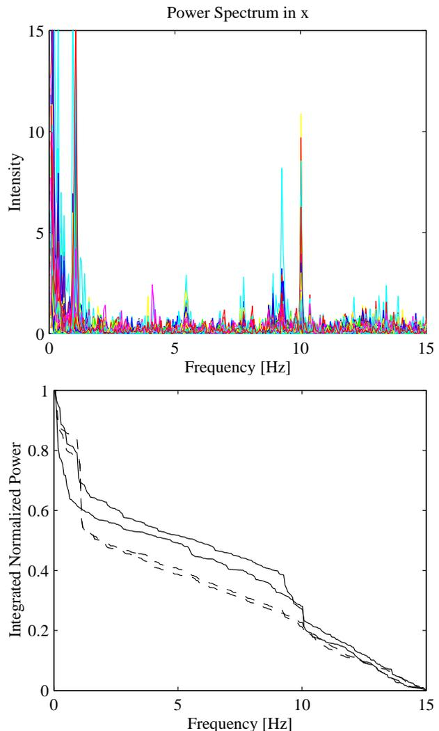
Figure 1: Transverse power spectrum and integrated part. The beginning (solid) shows a 10 Hz line while at the end (dashed) of linac the 59 Hz (aliased to 1 Hz) is stronger.
