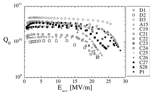
Figure 2: The quality factor as a function of accelerating gradient of those cavities measured in the vertical test stand, which reached more than 20 MV/m. The gradient of 5 cavities is limited by a quench in one cell, cavities C21, C22, C25, and S28 are limited by the available rf power.
