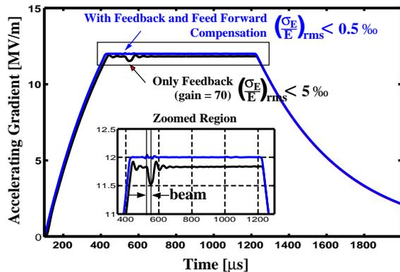
Figure 1: The accelerating gradient in a cavity as function of time during an rf pulse. The zoomed region shows the stability of the amplitude.
