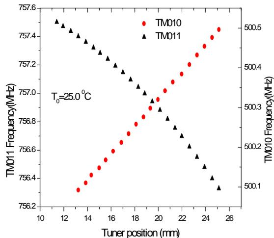
fundamental RF frequency, TM010 and the longitudinal HOM, TM011 mode as the tuner position changes. The cavity (C2) temperature was 25 °C.
