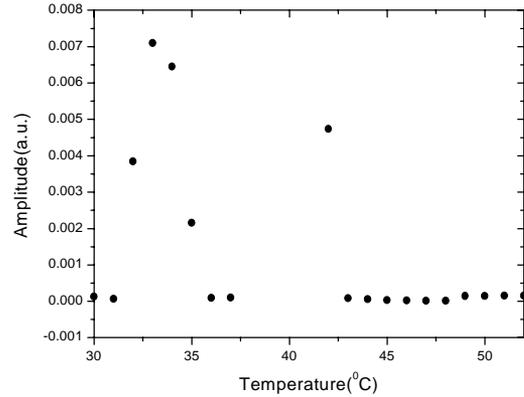
Figure 3. Measured amplitude of the instability induced by the mode TM011 as the cavity temperature was varied. Measurements was made by detecting amplitude of the corresponding synchrotron sideband.
