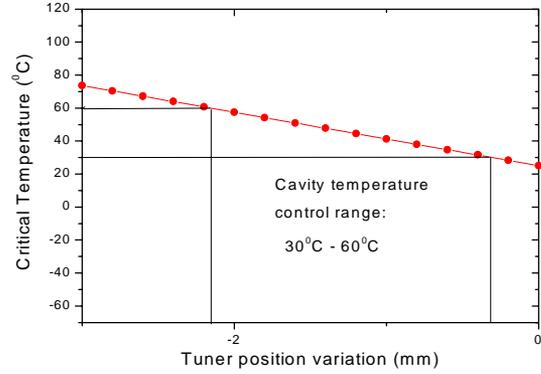
Figure 2. Critical temperature as a function of the tuner variation for C2 based on the Eq. (1).
