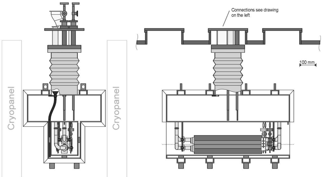
Fig. 7: Principal layout of the cryostat for an in-vacuum experiment.
