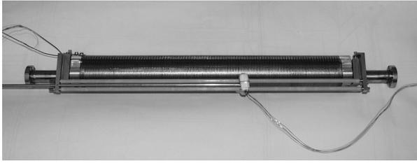
Fig. 4: One undulator half with the miniature Hall probe.
