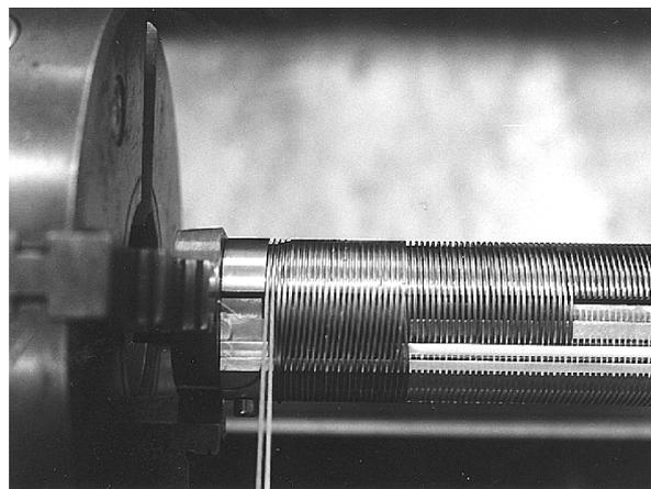
Fig. 3: Bifilar winding procedure of the undulator on a turn table.
