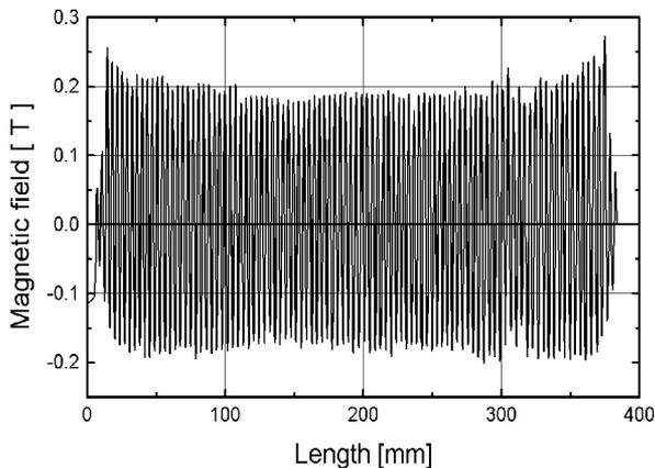
Fig. 5: Measured field of one undulator half.
