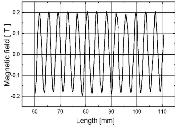
Fig. 6: Extended view of the magnetic field in the middle of the undulator.
