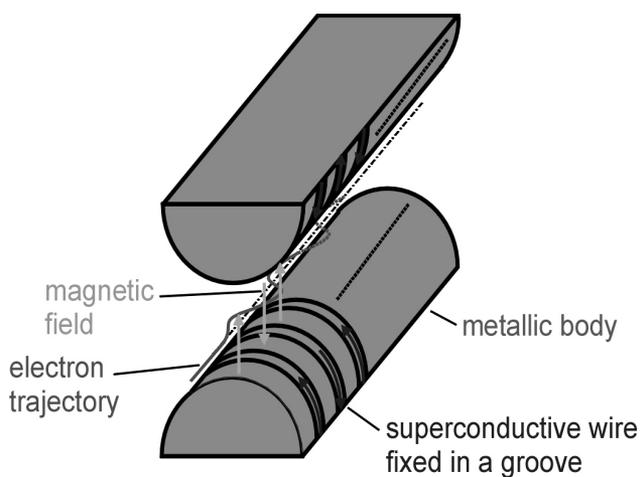
Fig. 1: Principal layout of the superconductive undulator.
