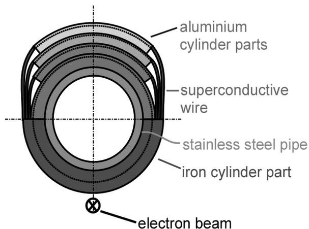
Fig. 2: The practical layout of the undulator.
