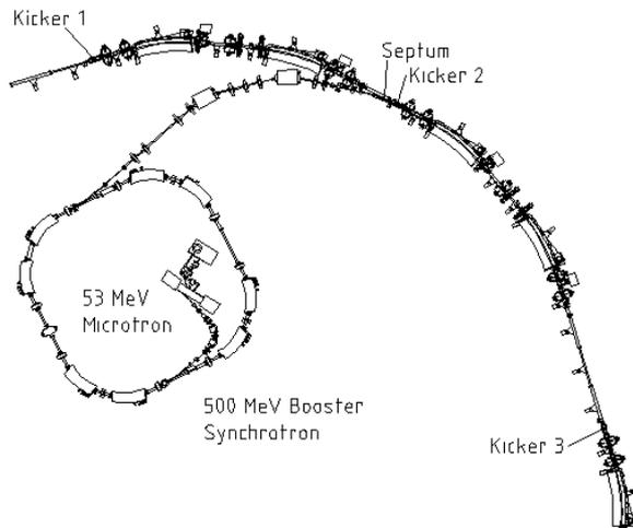
Figure 1: The injection geometry into ANKA
