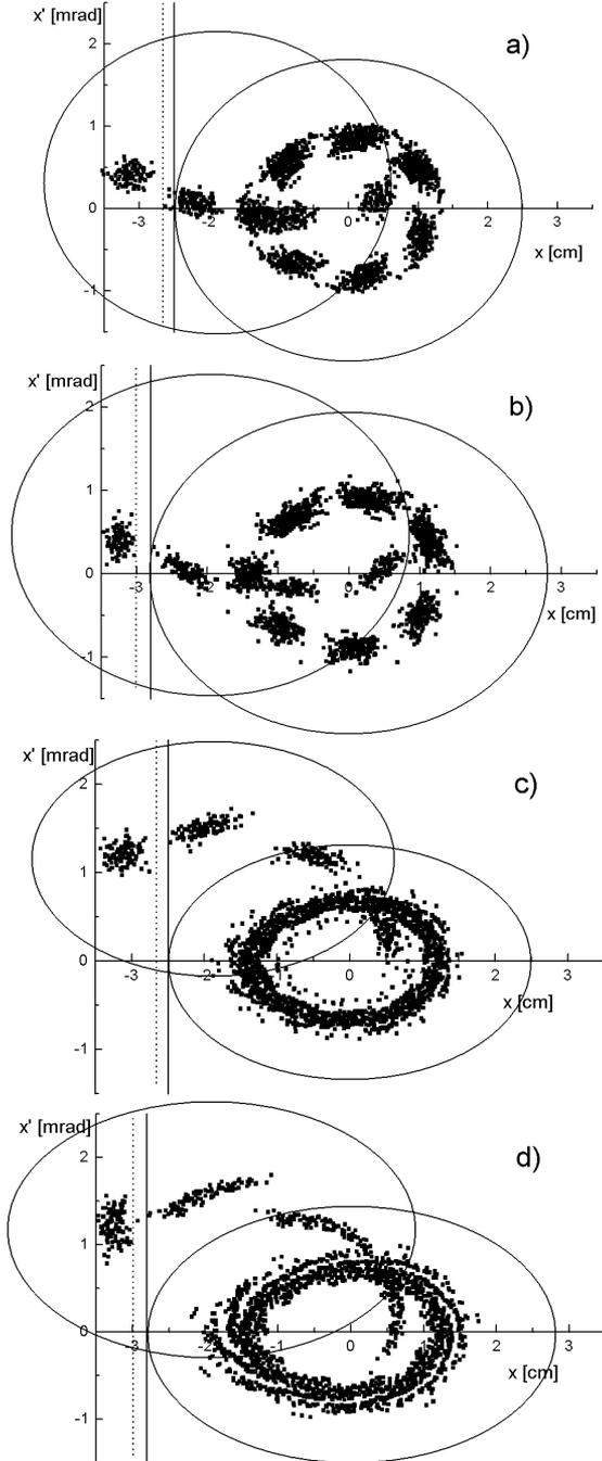
Figure 4: Injection into the storage ring ANKA for a) the f-optic in the case that the  $\beta$ -functions of the transfer line and the storage ring are identical = 14.5 m, b) as in a) but with a  $\beta$ -function of the transfer line of 7 m. c) as in a) but for the h-optic,  $\beta$ -functions are identical = 19 m and d) as in c) but the  $\beta$ -function of the transfer line is 7 m.
