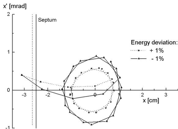
Fig. 6: The calculated energy acceptance for injection
