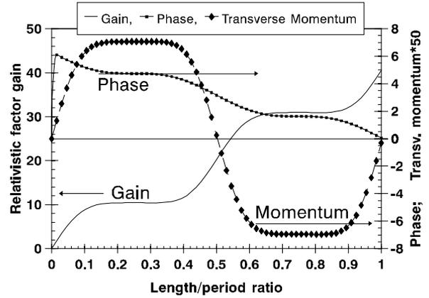
Figure 2. Energy gain  $\gamma(z)-\gamma(0)$ , transverse momentum  $\gamma\beta_x$  and resonant phase  $\varphi$  behaviour along the accelerator cell for  $n=1$ ,  $\lambda_s=1\mu\text{m}$ . Calculated effective undulator factor  $K_w=0.12$ .
