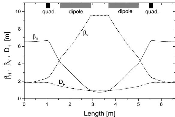
Figure 3: Betatron and dispersion functions in one super period of the booster synchrotron lattice (1/4 of the circumference) for  $Q_x=1.776$  and  $Q_y=1.173$ .
