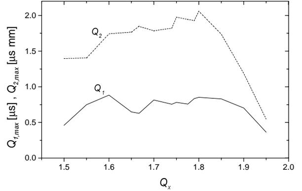
Figure 4: The maximum  $Q_1$  and  $Q_2$  values for several values of the horizontal tune  $Q_x$ . Realistic parameters:  $D_{x,bl}=0.2$  m,  $\epsilon_{x,m}=0.1$  mm mrad,  $\Delta p/p=0.2\%$ , and the effective septum blade thickness is 3.5 mm.
