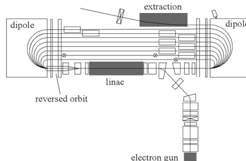
Figure 2: Schematic layout of the race track microtron.
