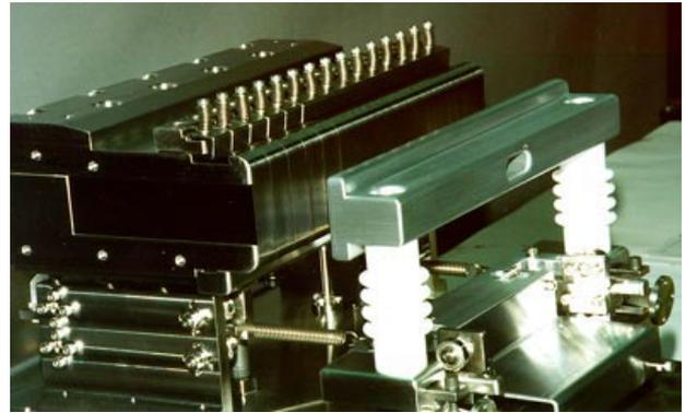
Figure 4: Fabricated electrostatic septum (ESS).
