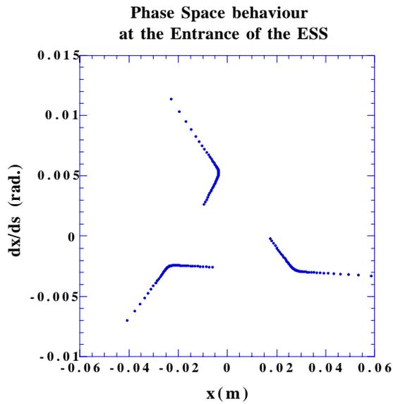
Figure 2: Beam behavior in the horizontal transverse phase space at the entrance of the ESS.
