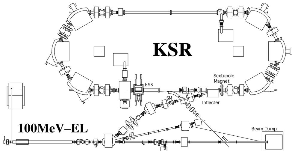
Figure 1: Beam extraction channel of the KSR stretcher mode and the injection line.
