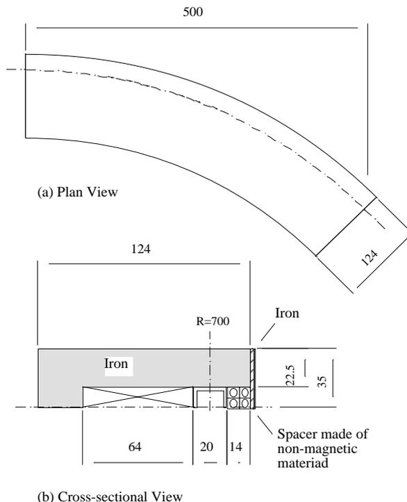
Figure 6: The septum magnet under design for KSR stretcher mode.
