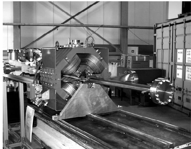
Figure 5: Prototypes of the quadrupole and the sextupole together with the dipole vacuum chamber. The straight section is equipped with a button beam position monitor.
