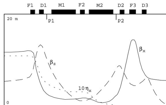
Figure 1. SIBERIA-2 optical functions at one half of cell.
