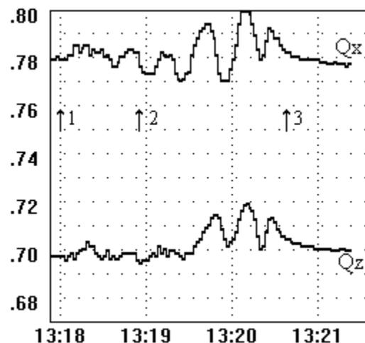
Figure 3. Typical betatron tune shifts during energy ramping. 1 - start at 0.45 GeV, 2 - 1 GeV, 3 - finish at 2.5 GeV.
