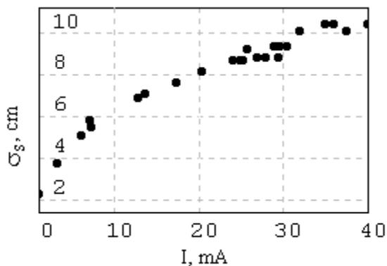
Figure 2. Dependence of longitudinal rms beam size on electron current in single-bunch mode.
