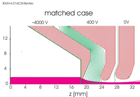
Figure 5: Plot of the beam trajectories for the matched case calculated with IGUN.
