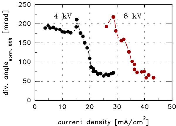
Figure 2: IGUN calculations of the divergence angle as function of the current density.
