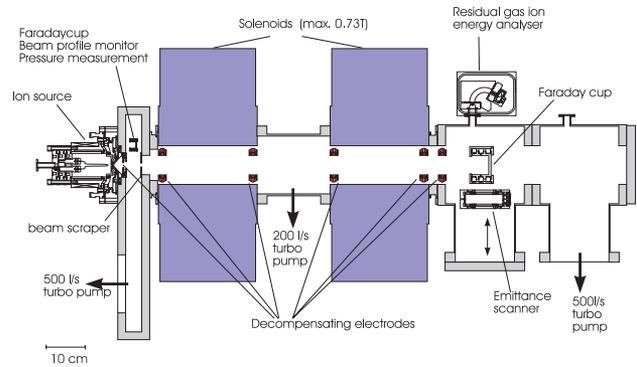
Figure 6: Schematic drawing of the experimental set-up of the Frankfurt LEBT line.
