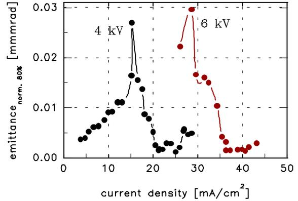
Figure 3: IGUN calculations of the emittance as function of the current density.
