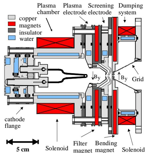
Figure 1: schematic drawing of the ion source.
