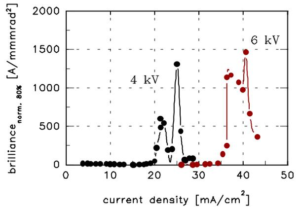
Figure 4: IGUN calculations of the brilliance as function of the current density.
