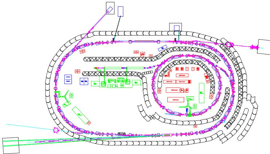
**Fig. 1:** Layout of the DELTA. FELICITA I is located in the northern superstraight. Two FEL beamlines are available to probe the radiation coupled out through upstream and downstream mirror.
