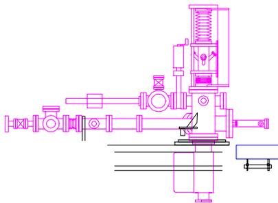
Fig. 2: Sketch of the FEL mirror vessel. The beam is entering the vessel through the beam pipe, coming from the left. The mirror can be pulled up by about 10 cm, and then be manipulated or changed through a gate system
