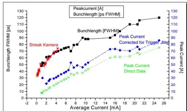
Fig. 4: Measurement of bunch length and peak current with a fast photodiode and a streak camera, respectively.
