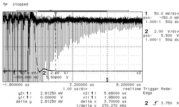
**Fig 5:** Ring down of the stored emission in the optical cavity. The electron beam was killed using a kicker magnet.
