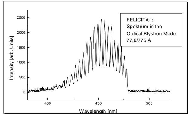
Fig. 3: Spectrum of the FELICITA I undulator in the optical klystron mode. The quality of this spectrum is reduced due to insufficient alignment of the pinhole.
