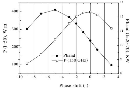
Figure 6: Computed power on the 50th harmonic (150 GHz) and total band power vs the phase shift between LINAC and PMS. The phase shift is defined respect to the value that maximises Pband.  $E_{\text{PMS}}=0.6 E_{\text{linac}}$ .
