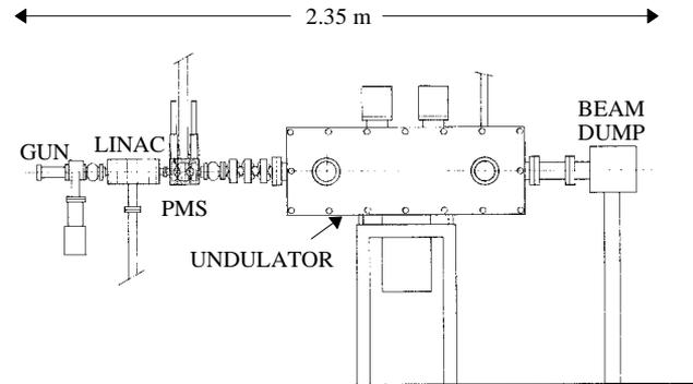
Figure 3: Experiment layout
