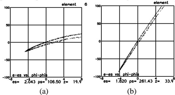
Figure 4: Computed phase-space distribution (a) at linac output (b) at PMS output
