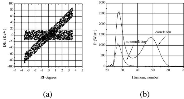
Figure 1: (a) correlated and uncorrelated energy-phase distributions (b) relative CSE power vs the harmonic number  $l$  of the fundamental frequency  $\nu_{RF} = 3$  GHz.
