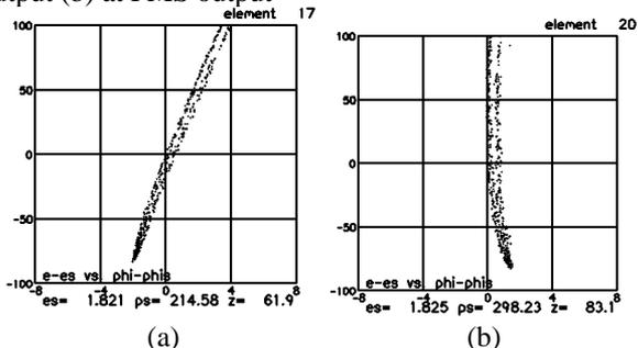
Figure 5: Computed phase-space distribution (a) at wiggler input (b) at the center of the wiggler
