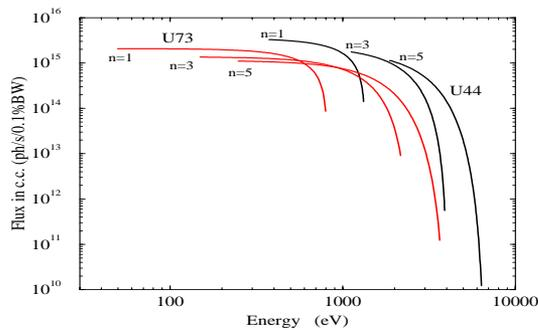
**Figure 2.** Spectral flux in central cone of LLS undulators U73 and U44.
