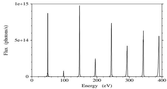
**Figure 3.** Spectral flux of U73 undulator at 2 cm gap in 100  $\mu$ rad in each direction
