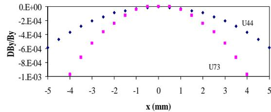
**Figure 7.** Relative transverse field uniformity of the LLS undulators at a gap of 5 cm.
