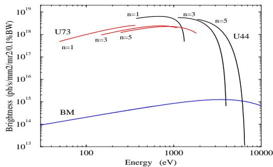
**Figure 1.** Spectral brightness of LLS undulators U73 and U44 compared with the bending magnet brightness.
