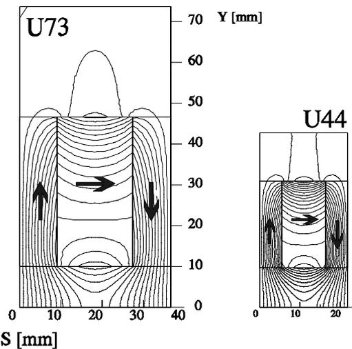
**Figure 5.** Basic cell of the U73 and U44 undulators.
