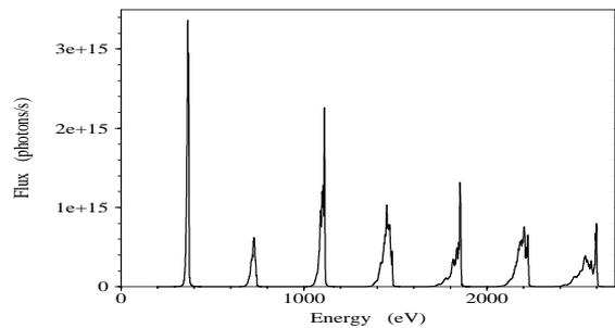
**Figure 4.** Spectral flux of U44 undulator at 2 cm gap in 100  $\mu$ rad in each direction.
