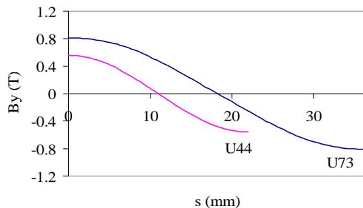
**Figure 6.** Field profile along the beam path for the U73 and U44.
