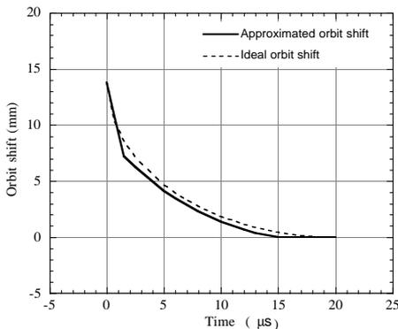
Figure 2: Actual waveform of the orbit shift bump magnet approximated to Equation (1)
