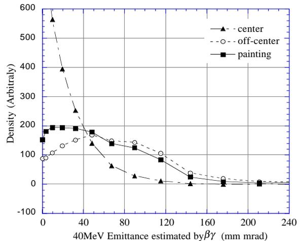
Figure 6: Particle density in the horizontal phase plane estimated from the transvers profiles.
