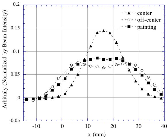
Figure 5: Particle distributions in the horizontal real plane measured by multi-wire profile monitor on the 500 MeV extracted beam line.
