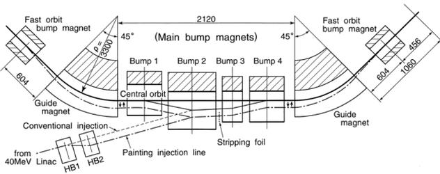
Figure 1: Charge-exchange injection system for phase space painting
