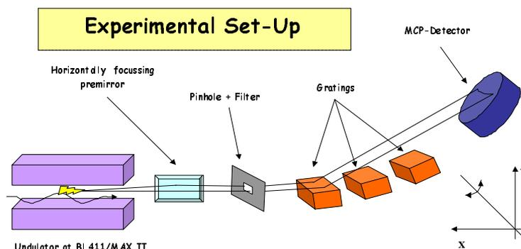
Figure 1: Experimental setup of the beamline during the characterisation.
