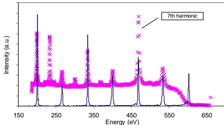
Figure 3: Measured and calculated undulator spectra at 25 mm gap using grating 3. Not corrected for transmission functions and detector sensitivity (x - measured, solid line - simulated).
