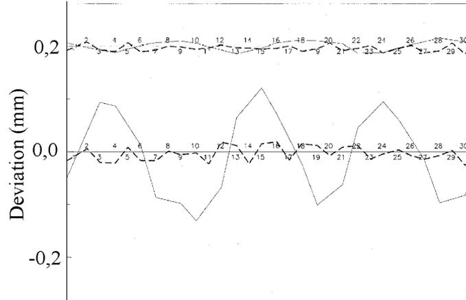
Figure 2: Electron beam position with closed undulator. (bottom - before correction, top - after correction. Dashed line - horizontal, solid line - vertical)
