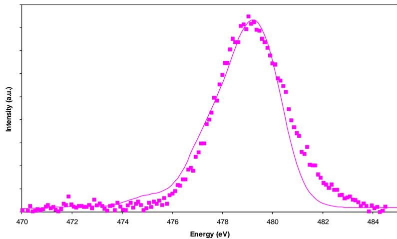
Fig 5. The 8<sup>th</sup> harmonic at 24 mm gap, using grating 1 with an energy spread of 0,07%. (dots - measured, solid line - simulated)
