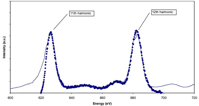
Figure 4: Harmonic 11 and 12 for 23,5 mm gap with grating nr1. High current and energy spread 0,22%. (dots - measured, solid line -simulation)
