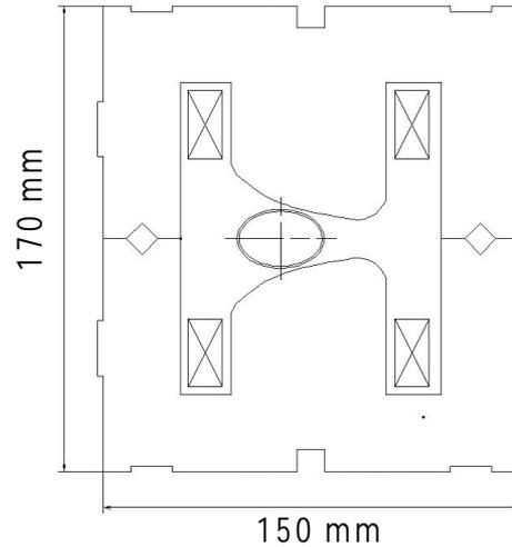
**Figure 3: Cross-section of a BF magnet with the 30x20 mm<sup>2</sup> vacuum chamber. The pole profile provides the combined (dipole plus quadrupole plus sextupole) magnetic field.**
