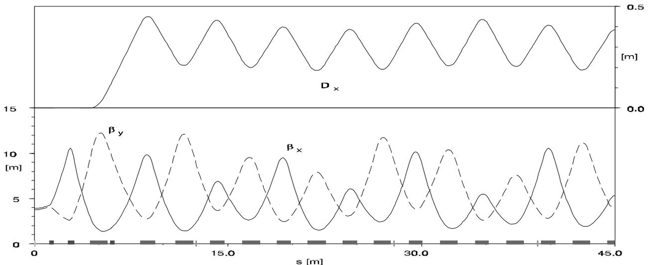
**Figure 4: Optical functions for 1/6 of the booster, from center of straight to middle of arc.**
