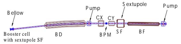
**Figure 2: Layout of one FODO cell with 2 combined function magnets (BD and BF), two steerers (CX and CY) and one sample sextupole (SF).**
