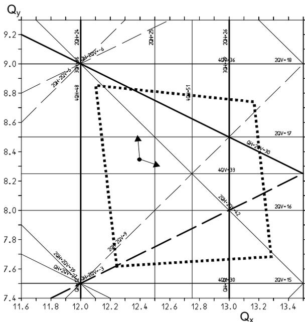
**Figure 5: Tune diagram, showing the working point (12.39, 8.35), with the change produced by a 1% gradient error in BD, BF (arrows), the accessible region with the three quadrupole families (dotted line), and the four major resonances (thick lines).**
