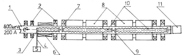
Figure 7: The experimental setup scheme on the base of LIA-3000: 1) injector exit; 2) magnetic field coils; 3) travelling wave tube; 4) waveguide; 5) magnetron; 6) magnetic solenoid; 7) first accelerating gap; 8) linear induction accelerating sections; 9) second accelerating gap; 10) corrugated waveguide; 11) diagnostic chamber.
