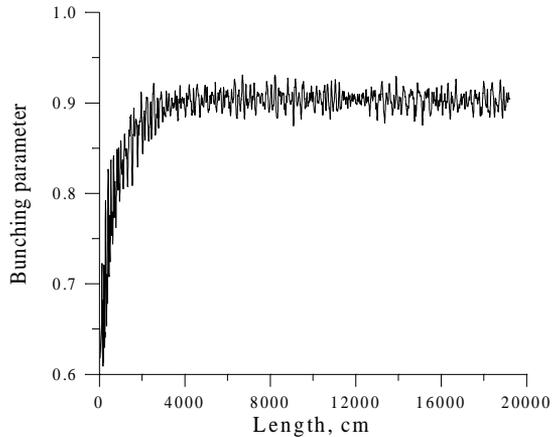
Figure 5: The bunching parameter versus the distance for continuously distributed driver parameters.
