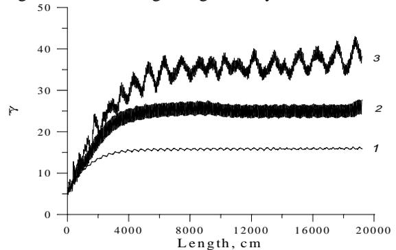
Figure 3: The electron mean energy versus the distance for: 1 - continuously distributed driver parameters; 2 - discrete periodic cells, 3 - discrete cells with narrow accelerating gaps.
