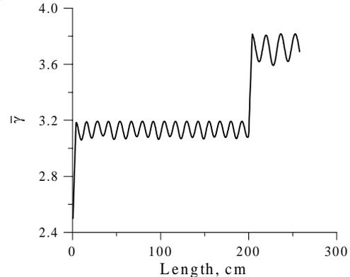
Figure 8: The electron mean energy versus the distance for LIA-3000 parameters.
