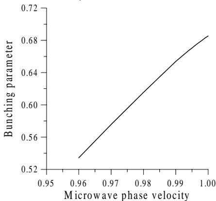
Figure 2: Dependence of the bunching parameter on the unloaded waveguide phase velocity  $\beta_{ph}$ .
