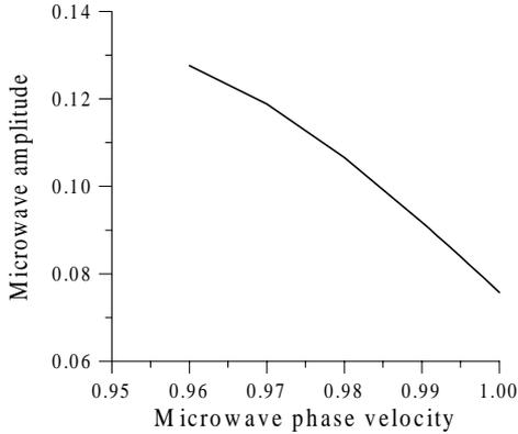
Figure 1: Dependence of the microwave amplitude  $a_{max}$  on the unloaded waveguide phase velocity  $\beta_{ph}$ .
