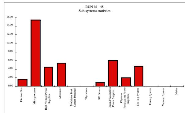
Figure 2: Downtime statistics by subsystem. The run 42 SF6 leak has been excluded to highlight the other fault sources.
