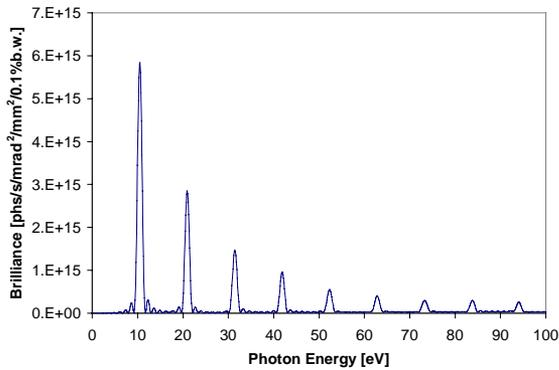
Fig. 4: Brilliance spectrum of APPLE-8 undulator. Circular polarization mode.
