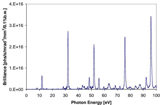
Fig. 6: Brilliance spectrum of a new QPU.  $r=1.4$ ,  $\eta = \sqrt{15}$ .
