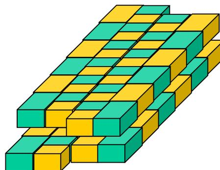
Fig.1: Schematic drawing of magnet configuration of APPLE-8. Finite magnet row phase case.
