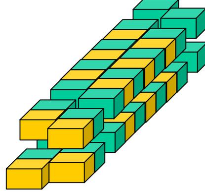
Fig. 3: Schematic drawing of Elliptically Polarizing QPU in new scheme.
