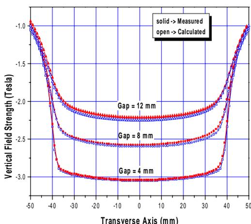
Figure 4: The measured and calculated field profiles along the transverse direction at different gap widths.
