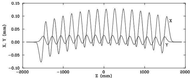
Figure 5. Simulated electron trajectory in the EEW after external correction of the field integral errors, with  $I_H = 300$  A,  $I_V = 150$  A.
