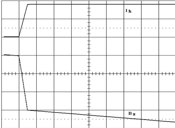
Figure 6. Horizontal current and field in the trapezoidal mode. Horizontal div. = 10 ms.
