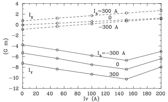
Figure 3. Variation of 1st field integrals with current.
