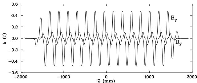
Figure 2. Measured field distributions in the EEW with  $I_H = 300\ \text{A}$ ,  $I_V = 150\ \text{A}$ .
