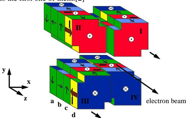
Figure 1: One period of magnets: The magnet blocks can be located at four quadrants (I, II, III and IV) and four quarter periods (a, b, c and d). The vendor marks the broad arrows showing the principal field direction and the series numbers which were indicated by small bars.
