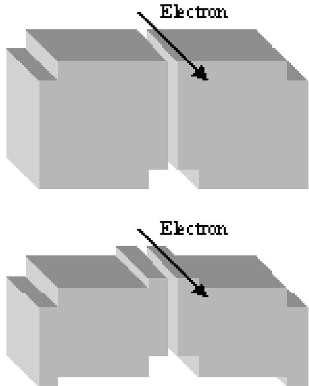
Figure 2: The prototype and new design of the magnetic blocks.
