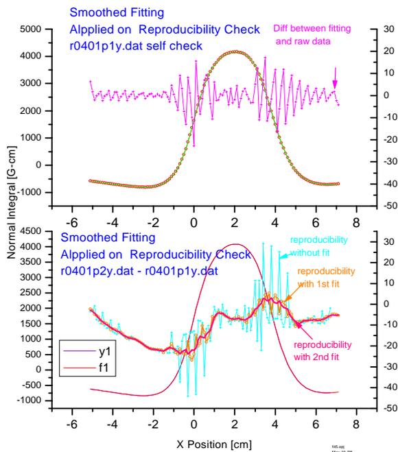
Figure 4: After fitting process, the trigger errors can be cured. From the upper graph, one can see the obvious regular trigger error due to subroutine calling. The lower graph shows that after two step fitting, the remaining
