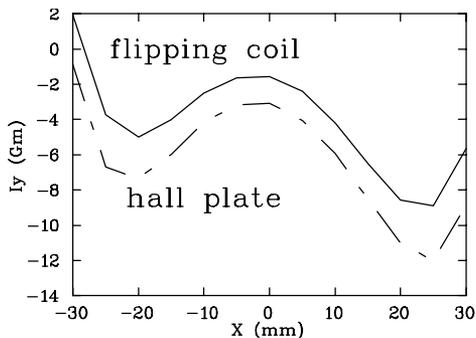
Fig.5 Field integral variation at a distance of 10 mm from the poles, measured with the flipping coil and hall plate.
