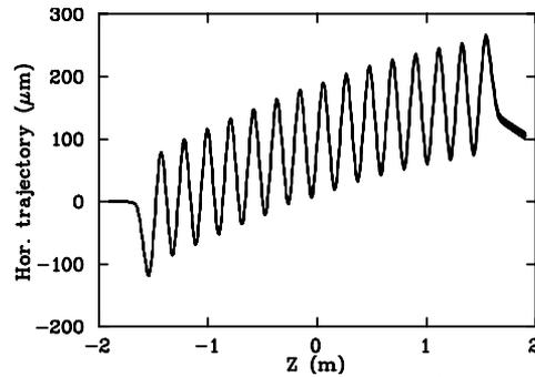
Figure 3: 8 trajectories calculated from magnetic measurements in the EEW.
