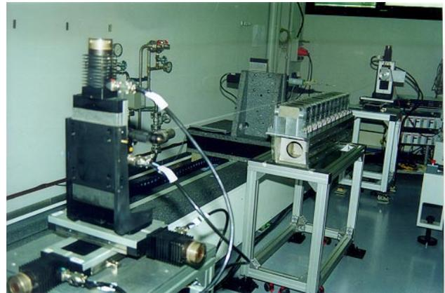
Fig.4 The stretched wire and hall plate benches.
