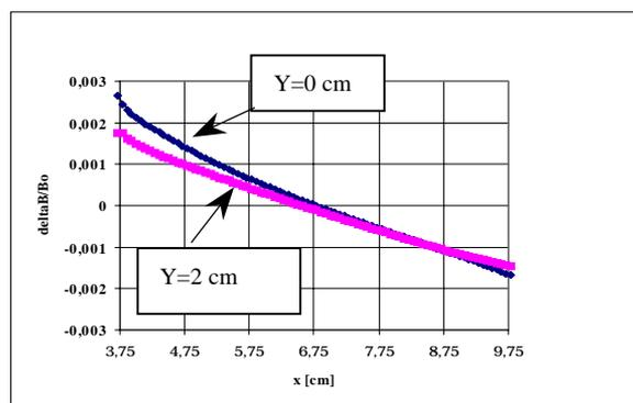
Figure 3: Relative magnetic field distribution in the kicker aperture for different y-values.
