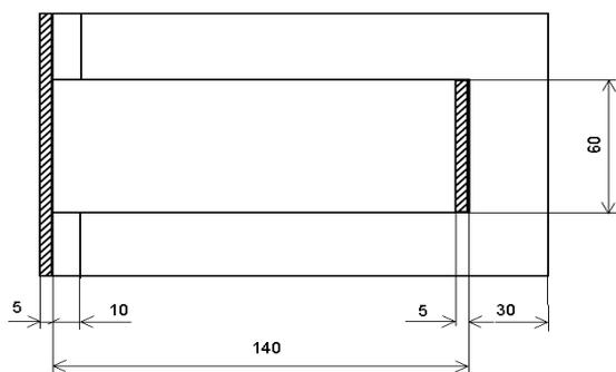
Figure 2: Schematic drawing of the kicker magnet.
