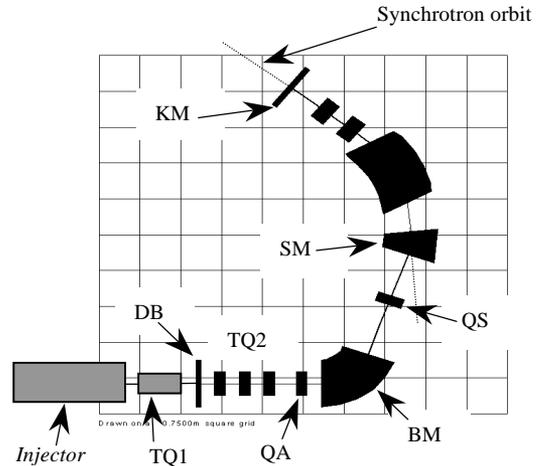
Figure 1: General layout of the injection beamline.
