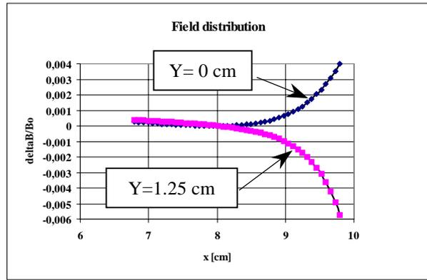
Figure 6: Relative magnetic field distribution for different y-values.
