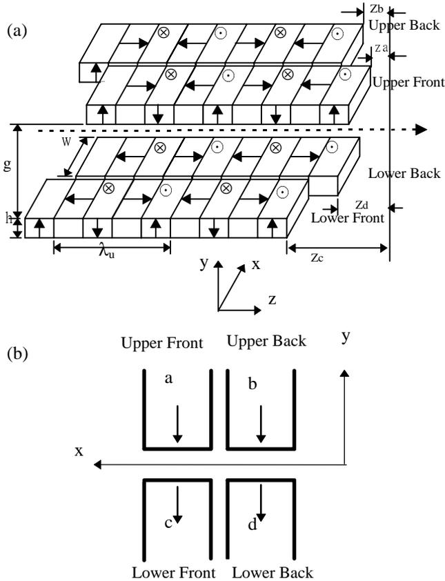
Figure1: (a) The schematic magnetic array structure of the EPU. (b) Location relation between a, b, c, and d four rows in the x-y plane.
