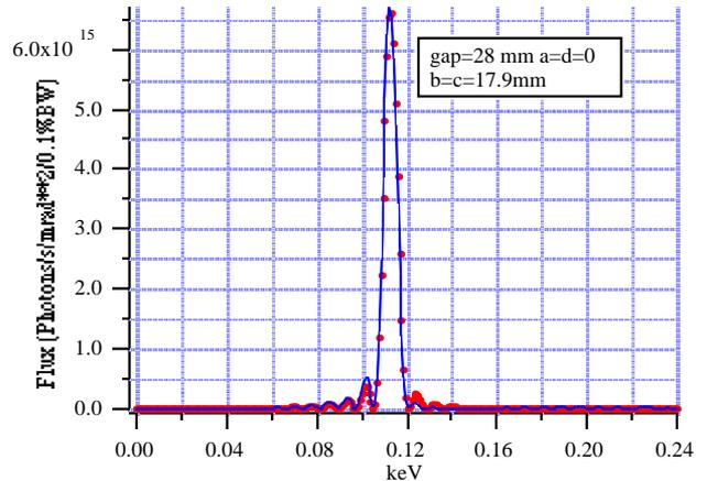
Figure2: Photon flux was calculated at the circularly polarized radiation (mode 1).
