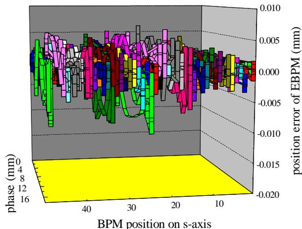
Figure 4: The electron orbit deviation is measured on mode 1. The phase change can get the optimize polarization rate in dynamic tuning.
