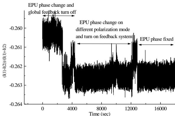
Figure 5: The photon flux variation when the EPU phase was operated at different polarization mode. Where  $I(1)$  and  $I(2)$  are the photon current of the two PBPMs.
