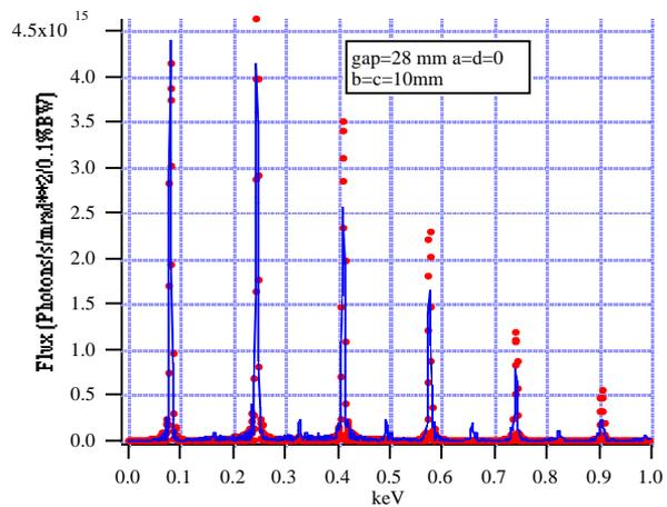
Figure3: Photon flux was calculated at the elliptically polarized mode (mode 1).
