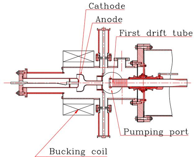
Figure 2: Schematic of the 10 A electron gun.
