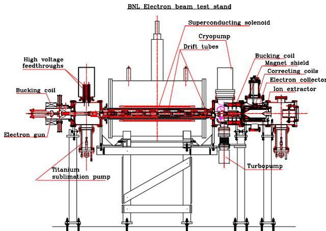
Figure 1: Layout of the electron beam test stand.
