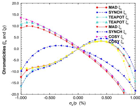
Figure 4: A Comparison of the Chromaticity Dependence on Momentum between four codes MAD, SYNCH, TEAPOT, and COSY.
