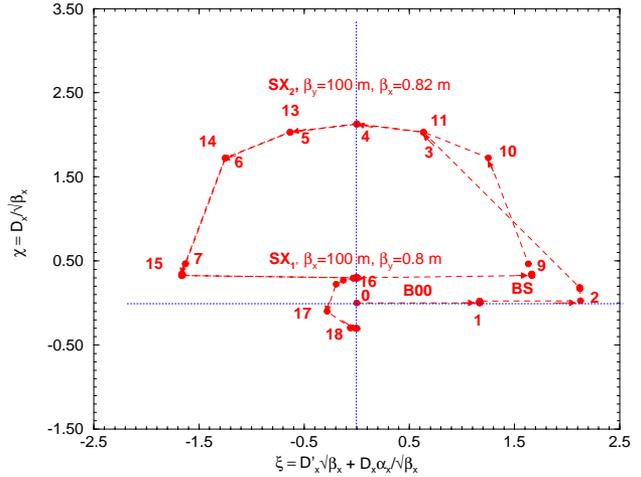
Figure 2: The local chromatic correction in normalized dispersion space.
