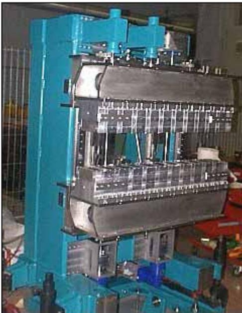
Figure 5. Photograph of a fully assembled multipole wiggler.
