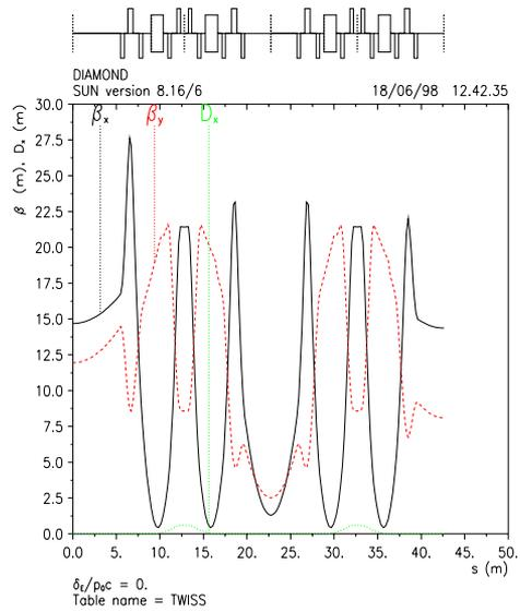
Figure 1: Twiss and dispersion functions for one octant.
