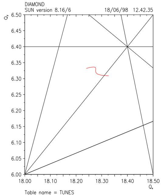
Figure 3: Working diagram showing tune shifts up to  $\pm 3\%$ ; resonances up to order 5 are plotted.
