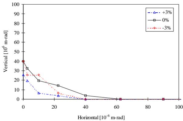
Figure 5: Racetrack Lattice - dynamic acceptance for on-momentum and  $\pm 3\%$  off-momentum particles (tracked with MAD for 200 turns using 4<sup>th</sup>-order Lie method).
