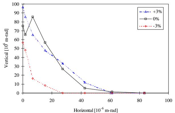
Figure 4: Dynamic acceptance for on-momentum and  $\pm 3\%$  off-momentum particles (tracked with MAD for 200 turns using 4<sup>th</sup>-order Lie method [4]).
