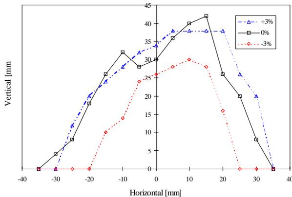
Figure 6: Dynamic aperture for on-momentum and  $\pm 3\%$  off-momentum particles (tracked with MAD for 200 turns using 4<sup>th</sup>-order Lie method), observed at centre of long straight section ( $\beta_x = 14.7$  m,  $\beta_y = 12.0$  m).
