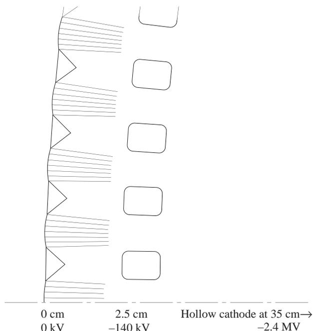
Fig. 3. Model for concentric annular preaccelerator grids.
