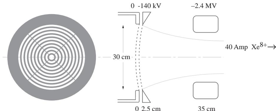
Fig. 2. High perveance extractor concept for laser ion source with magnetic bucket, showing concentric annular grids.
