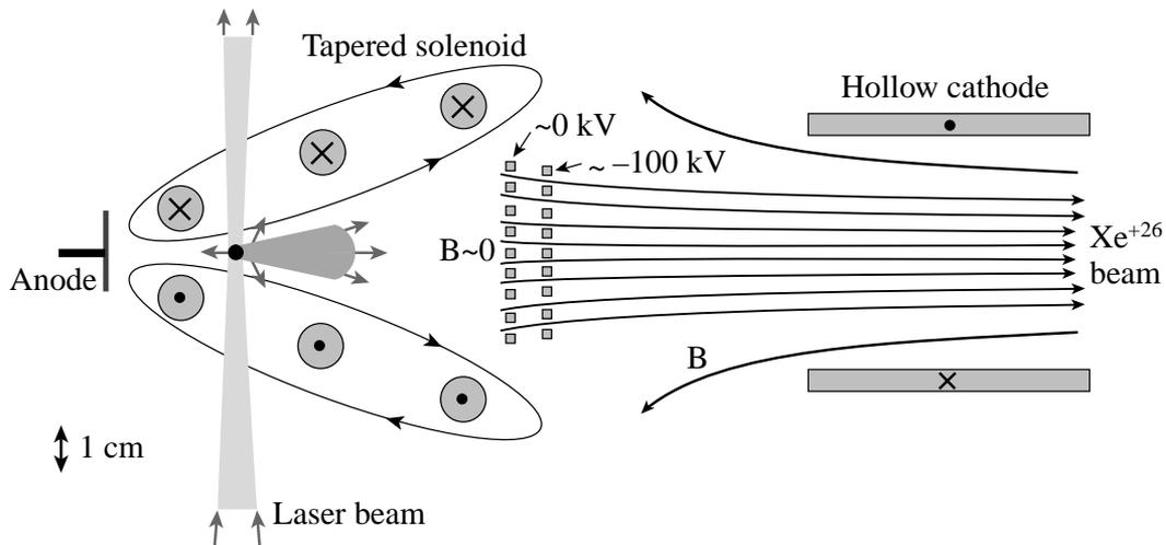
Fig. 1. A conceptual method of extracting highly-charged ions created by a short-pulse laser. Frozen Xenon targets  $\sim 10 \mu\text{m}$  in radius are prepulsed by a low energy laser and expanded well below the critical density before the main pulse. Typical numbers for the main laser:  $0.5 \mu\text{m}$ , 100 fs, 1 petawatt. The tapered solenoid field directs ion flow toward the concentric annular extractor grids, which are adjusted radially to control beam aberrations.
