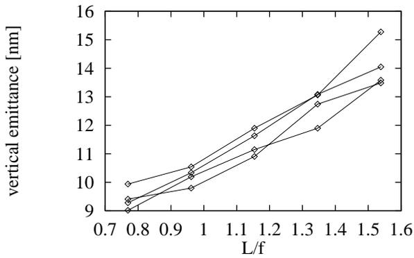
Figure 5: The emittance after  $10^6$  s of ground motion using one-to-one feedbacks for different—initially perfect—lattices. The different curves correspond to different focal lengths  $f$  ranging from 0.975 to 1.4625 m.
