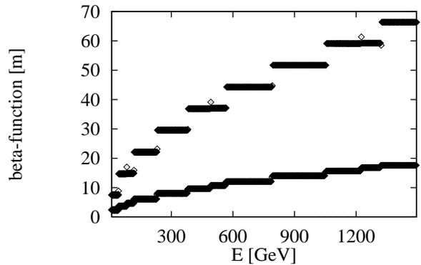
Figure 1: The beta-function along the 3 TeV-linac.
