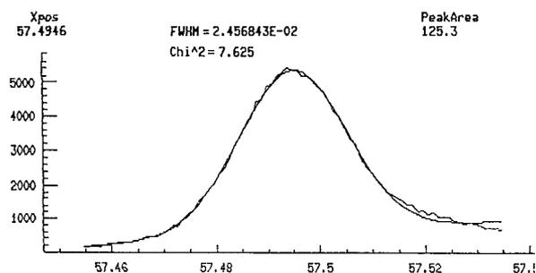
Figure 1: Rocking curve for C<sub>2</sub>. Abscissa in degree.
