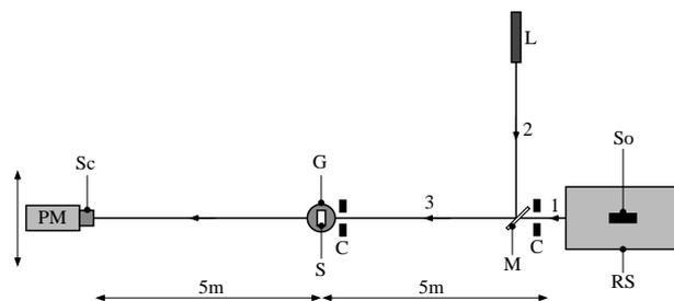
Figure 2: The Stuttgart  $\gamma$ -diffractometer set-up. So:  $^{137}\text{Cs}$  radioactive source, RS: radiation shield, C: collimators, L: laser light source, M: mirror, G: goniometer, S: sample, Sc: BGO scintillator, PM: photomultiplier, 1:  $\gamma$  beam, 2: laser light, 3:  $\gamma$  beam and laser light.
