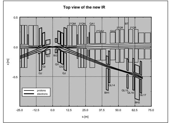
Figure 2: IR layout (right side)
