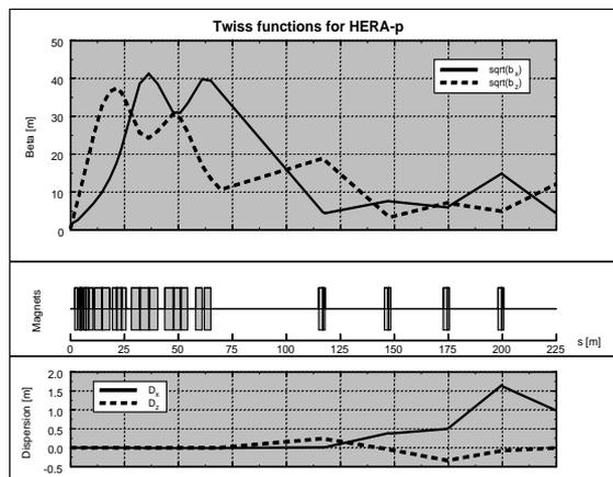
Figure 3: Proton ring Twiss functions at the new IP.
