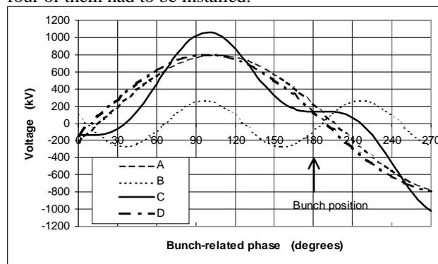
Figure 1: Design voltages in the double RF system. A: main cavity voltage with the passive system tuned, B: voltage in the passive cavity system, C: total voltage, D: main cavity voltage with the passive system detuned.
