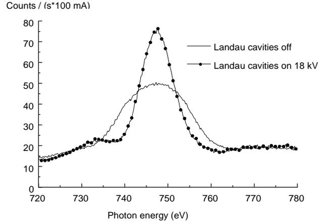
Figure 3: The effect of the Landau cavities on a high harmonic of undulator 411.
