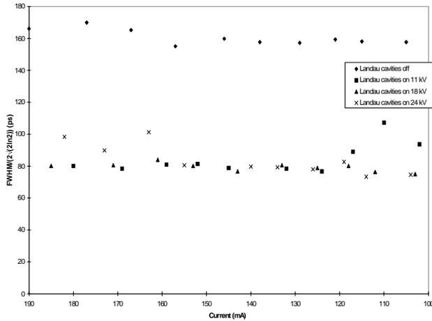
Figure 4: Bunch lengths, as measured with the OSO, with and without Landau cavities.
