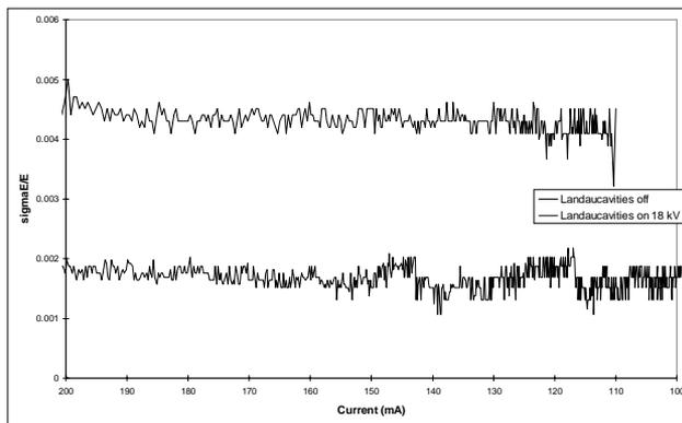
Figure 2: The beam energy spread versus beam current with and without Landau cavities.
