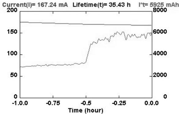
Figure 5: Beam current, and beam current times beam lifetime, versus time. The Landau cavities are tuned to 18 kV, at -0.5h. The measurement is done with 10% emittance coupling.
