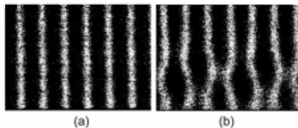
Figure 2. Snapshots taken every 4  $\mu\text{sec}$  before and after the turn-off of the ion pumps. Total time span in horizontal direction is 25  $\mu\text{sec}$  (6.4 mm in spatial unit), and 500 nsec in vertical direction. a) Snapshots taken at nominal condition. Very weak oscillation was observed at the very tail of the bunch train. b) After ion pumps were turned off, the snake-tail oscillation at the tail is clear.
