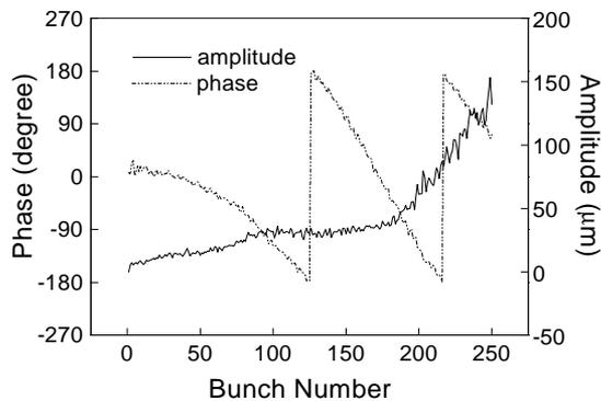
Figure 4. The phase advance and amplitude of bunch train oscillation plotted from an SBPM data taken before the He injection. Phase advance per bunch is  $\sim 2\pi/95/\text{bunch}$  at the tail, which agrees with the frequency of 5.4 MHz measured with the spectrum analyzer
