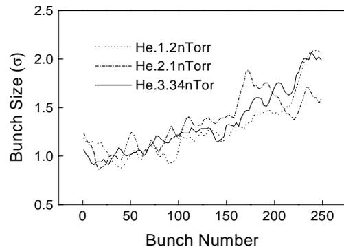
Figure 5. Bunch size measured along the bunch train for three different cases of 1.2 nTorr, 2.1 nTorr, and 3.34 nTorr showing the same growth pattern. Bunch sizes are normalized to the initial bunch size.
