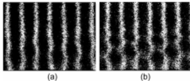
Figure 3. Two series of snapshots taken after He injection. a) Snapshots for 0.2 nTorr He, and b) for 3.34 nTorr He. The increase of the ion frequency from Figure 2b is manifest. The beam size blow-up at the tail is also clearly shown.
