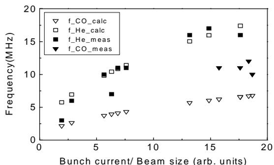
Figure 1. Ion frequencies measured and calculated with varying bunch current and bunch sizes.
