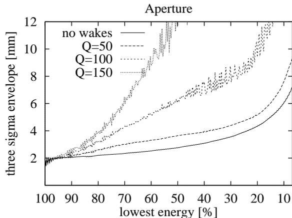
Figure 8: The beam envelope in the Decelerator with a one sigma offset for several different  $Q$ s.
