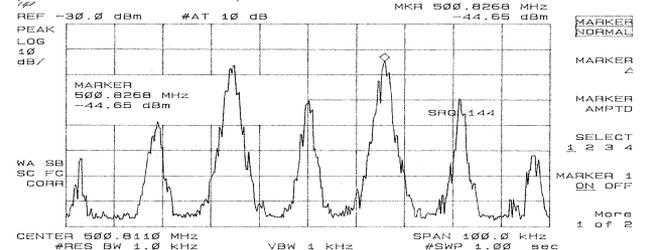
Figure 6: Mode cancellation breaks for a different filling pattern (6 bunches) (side band at -45 dBm).
