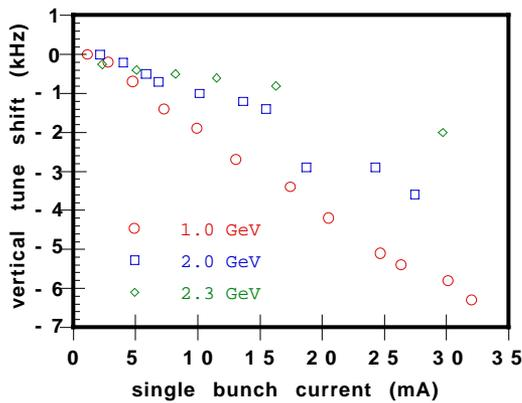
Figure 7: Variation of vertical tune with single bunch current at 3 different energies; 1 , 2 , 2.3 GeV
