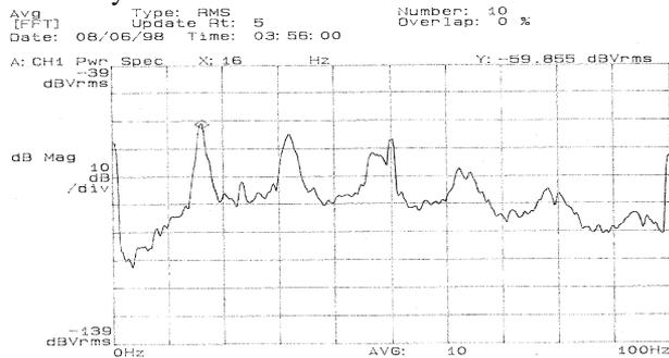
Figure 3: Low frequency beam spectrum in the absence of longitudinal but in the presence of strong TCBI excitation at 2 GeV and 130 mA.
