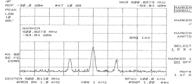
Figure 5: Mode cancellation for four bunches at 1 GeV (sideband at -94 dBm).
