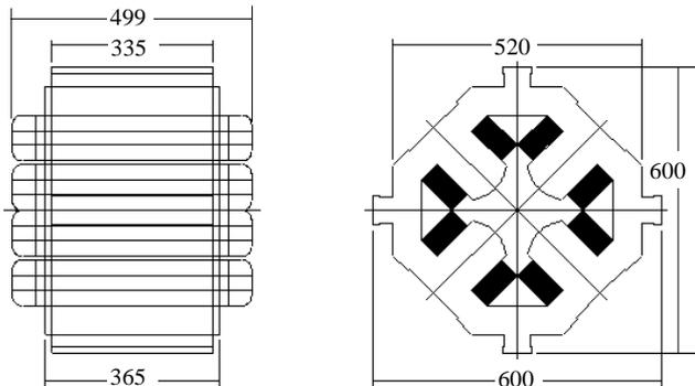
Figure 2: General layout of the quadrupole magnet
