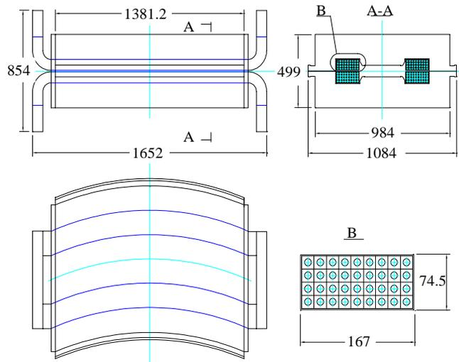
Figure 1: Technical design of the dipole magnet
