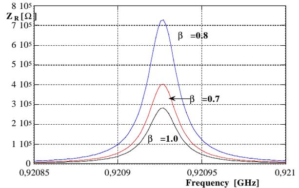
Figure 4: Longitudinal coupling impedance for various  $\beta$  around the first resonance.
