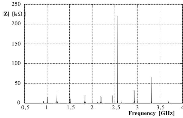
Figure 2: Longitudinal coupling impedance for a copper pill-box cavity for  $\beta$  equal 1.
