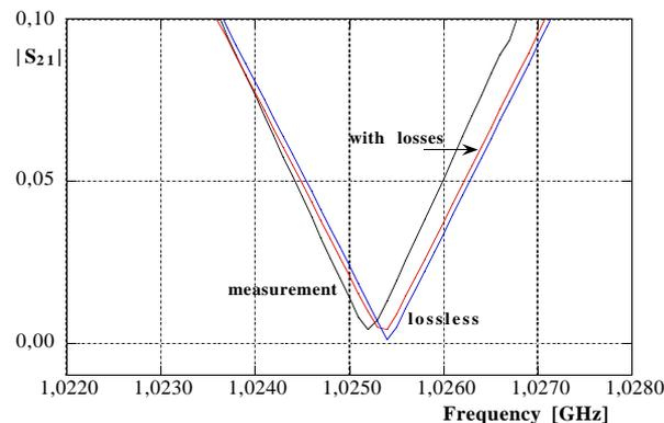
Fig. 7: Comparison between experimental and lossy/lossless simulations for the first resonance.
