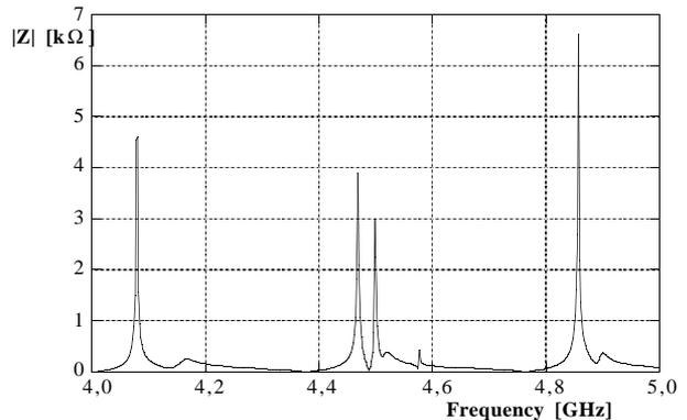
Figure 5: Longitudinal coupling impedance for a copper pill-box cavity for  $\beta$  equal 1, above the cut-off.
