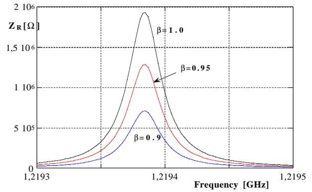
Figure 3: Longitudinal coupling impedance for various  $\beta$  around the second resonance.
