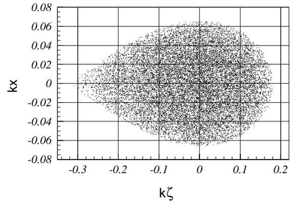
Fig. 1. Approximate stationary particle distribution in RF filed for  $\varphi_s = -1$ ,  $C_1 = 3.8$ ,  $k = \omega/v_s$ .
