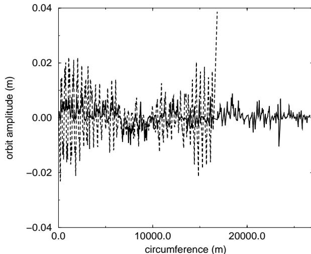
Figure 2: Unaided MAD tracking (dashed, big amplitudes) and tracking with threader (solid, small amplitudes), horizontal projection. The unaided particle hits the beam screen and is lost. The threaded particle amplitude stays below 11 mm over the full circumference.
