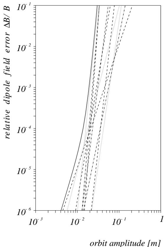
Figure 1: Relative field errors as a function of the radial distance from the zero orbit. Since the lower orders will be corrected, only the orders 4 to 15 are shown (12 and 14 are missing, see Table 1). The steeper a line, the higher the order. The bent curve at the left gives the total of all orders shown.
