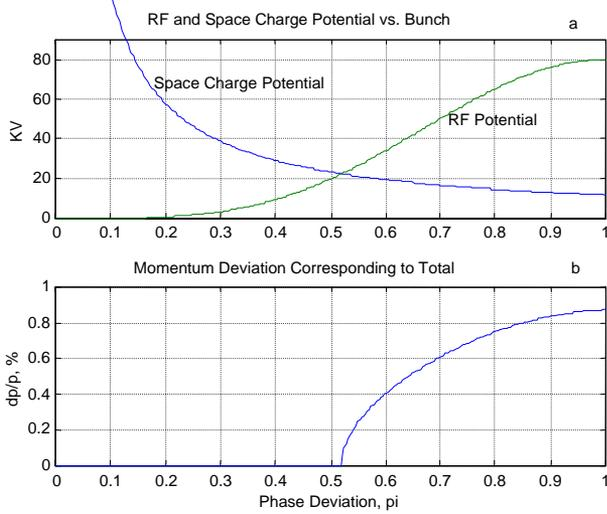
Fig.1. RF and Space Charge Potential
