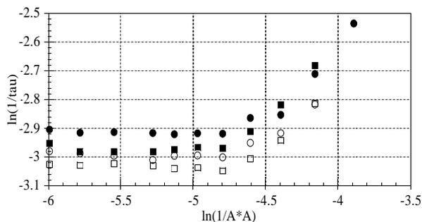
Figure 6: Comparison of the horizontal dynamic aperture measurements between the scenario with all the existing planar devices energised (white markers) and with also the EEW included (solid markers).
