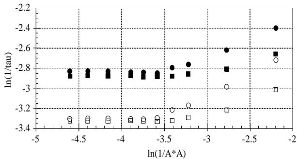
Figure 5: Comparison of the vertical dynamic aperture measurements between the bare lattice with sextupoles only (white markers) and with the EEW set to its nominal fields (solid markers).
