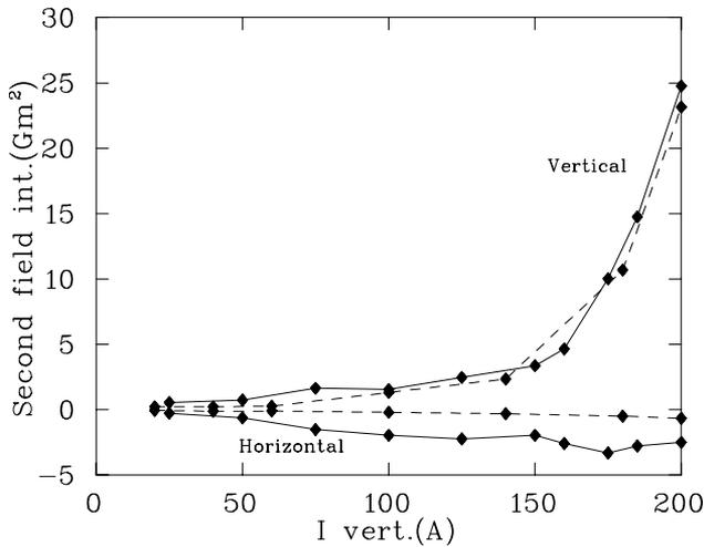
Figure 2: Horizontal and vertical second field integrals measured on the electron beam (solid lines) and in the magnetic measurement laboratory (dotted lines).
