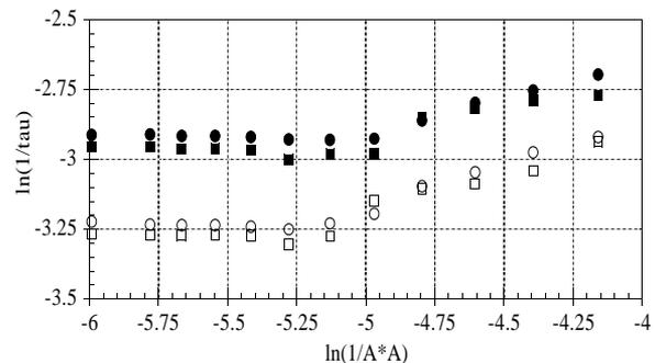
Figure 4: Comparison of the horizontal dynamic aperture measurements between the bare lattice with sextupoles only (white markers) and with the EEW set to its nominal fields (solid markers).
