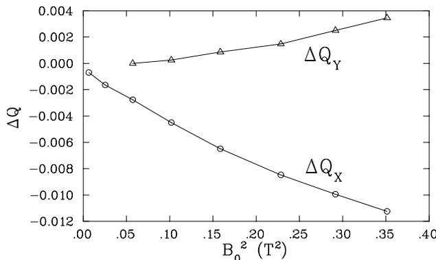
Figure 3: Measured tune shifts as a function of the square of the maximum on-axis vertical field.
