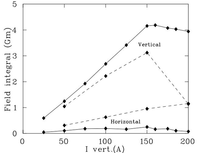
Figure 1: Horizontal and vertical first field integrals measured on the electron beam (solid lines) and in the magnetic measurement laboratory (dotted lines).
