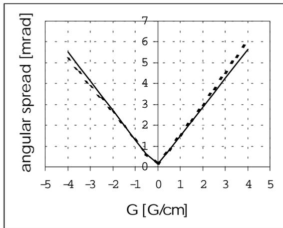
Fig.2. The dependence of angular spread of the electron beam on quadrupole gradient for section modified betatron.  $E=4$  MeV,  $B=1$  kG,  $I=0.1$  A. dashed line is the horizontal angular spread, solid line is vertical one.
