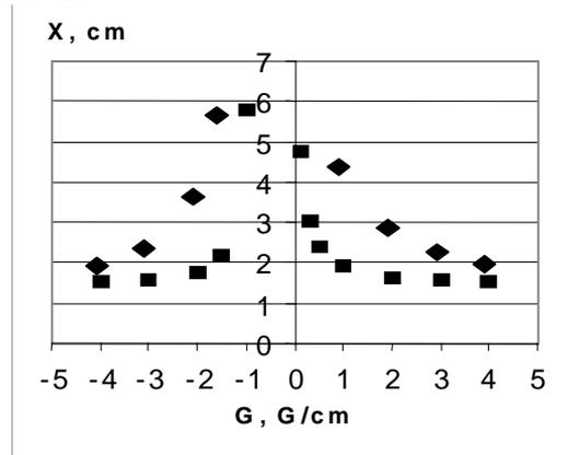
Fig.3. The dependence of horizontal coordinate on quadrupole gradient for modified betatron with quadrupole section.  $\blacklozenge$ - $\delta B_x/B_x \approx 10^{-2}$ ,  $\blacksquare$ - $\delta B_x/B_x \approx 10^{-3}$ , initial horizontal coordinate  $x_0=1.5$  cm,  $B=1$  kG,  $E=3$  MeV,  $I=0.2$  A.
