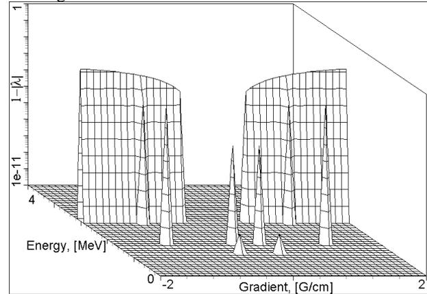
Fig.1. The electron beam instability islands for the MOBY structure when one straight kicker sections have no quadrupole coil.  $I=0.1$  A,  $B=1$  kG
