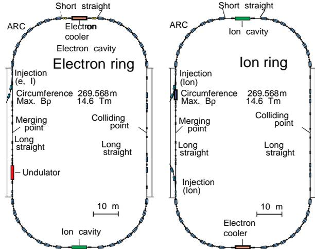
Fig. 1 Two rings in the DSR. 1a is an electron ring and 1b is an ion ring.
