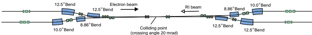
Fig. 2 Side view of the colliding section.
