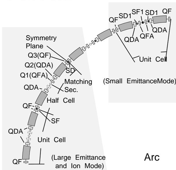
Fig. 3 Composition of the arc section.
