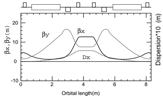
Fig. 4  $\beta$  and dispersion functions in the unit cell for S.E.M.
